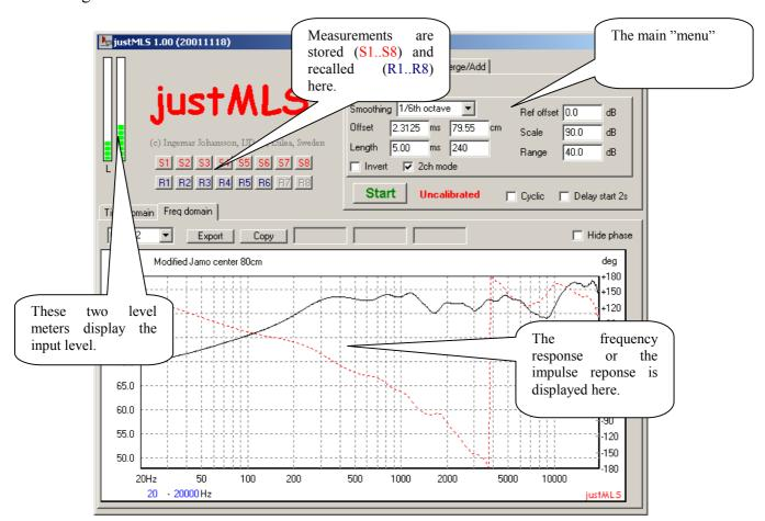
Up to eight different measurements can be stored in memory. The latest done measurement visible in the graphs is referred to as the current measurement. Two vertical bars display the input level.
