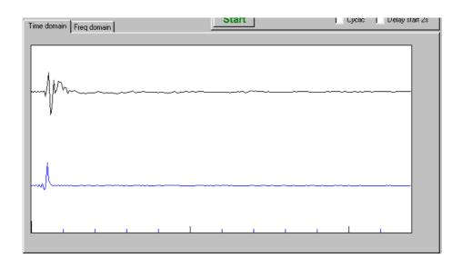
When the offset of the window is set appropriately it is high time to have a look at the frequency response. The length of the analysis is set such that as much of the room reflections are avoided still with the goal of at least some resolution in the lower frequency region. The
