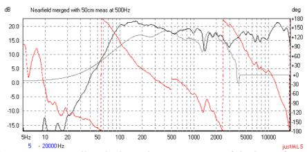
(500Hz). One may as well scale down the measurement of the lower frequency range, it is a matter of taste. The black graph is the merged response that one would get when the **Apply** button is pressed.
