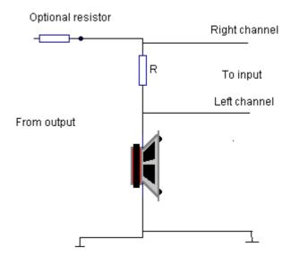
The recommended procedure is to select the input (preferably line input), calibrate the soundcard, set the levels and press the **Start** button. It is important to do a calibration as a very small difference between the channels may reflect largely on the impedance measurement.
