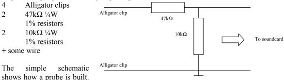
In cases with higher voltages it may be necessary to replace the  $47k\Omega$  resistor with a higher value (e.g  $470k\Omega$ ). The attenuation ratio is not critical as justMLS anyway cannot measure absolute values.
