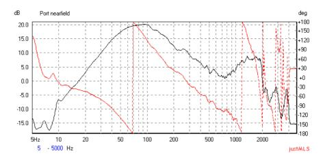
The driver and port measurements are stored in memory locations 1 and 2. The driver and port measurements are added by means of the Merge/Add menu (see fig below). The port measurement (red) is scaled down 8.6dB o that it matches the level of the loudspeaker unit (blue) below the port resonance. The thick black graph is the summed response. The **Apply**
