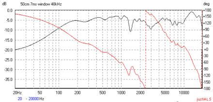
best choice this time is a 7ms window, see figure above. A 1/12<sup>th</sup> octave smoothing is applied to the measurement to make it look less noisy.
