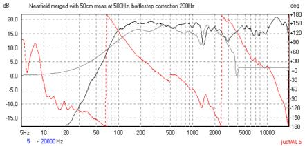
The phase response (red) shows a slight jump at the merge frequency (500Hz) that is not natural, we set the delay of the lower part to -138us and thus we get rid of the phase jump.
