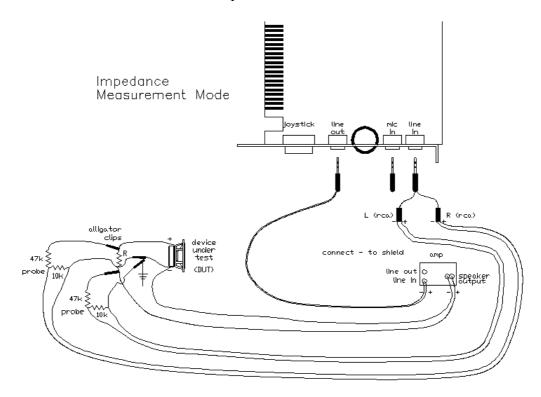
In some cases it is possible to use the line output from the soundcard, then an extra "optional resistor" of  $1k\Omega$  is also recommended. The connection of the left and right channels is not critical as justMLS will figure out the connection anyway.
